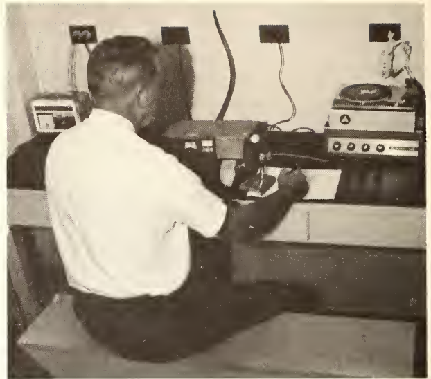
This 6-meter amateur band radio at West Point-Pepperell's Lanett Bleachery and Dye Works is part of plant's emergency communications system.
